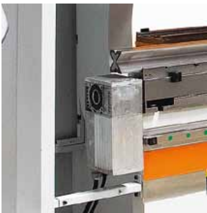
CNC Motorised Crowning System (*) CNC crowning system that communicates with the CNC controller, performs crowning automatically and enables the part to be at even bending angle at any given point. * Up to 400 TN optional. From 400 TN and above standard.
