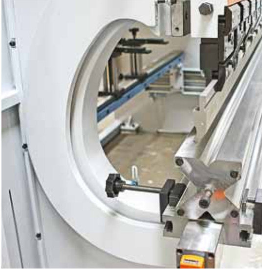
Throat (O) Special throat depths are offered up to 1500 mm for large bendings.
