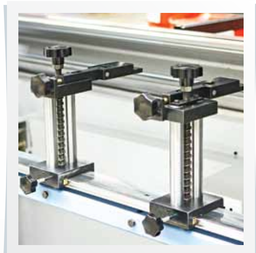
Backgauge Fingers (O) Specifically designed folding backgauge fingers.
