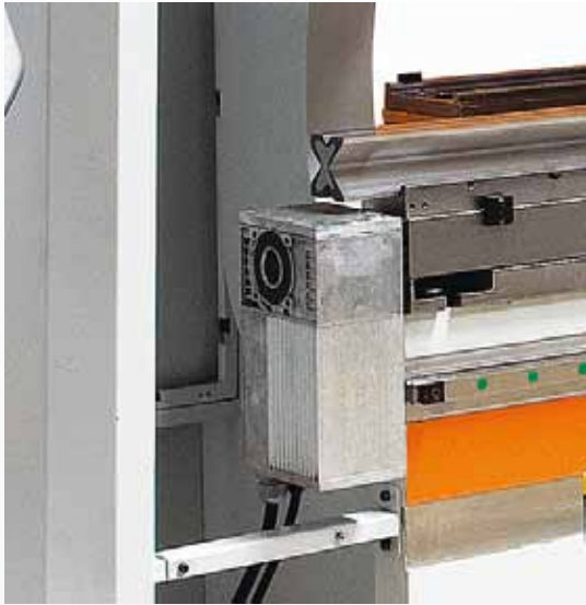
CNC Motorised Crowning System (S) CNC crowning system that communicates with the CNC controller, performs crowning automatically and enables the part to be at even bending angle at any given point.
