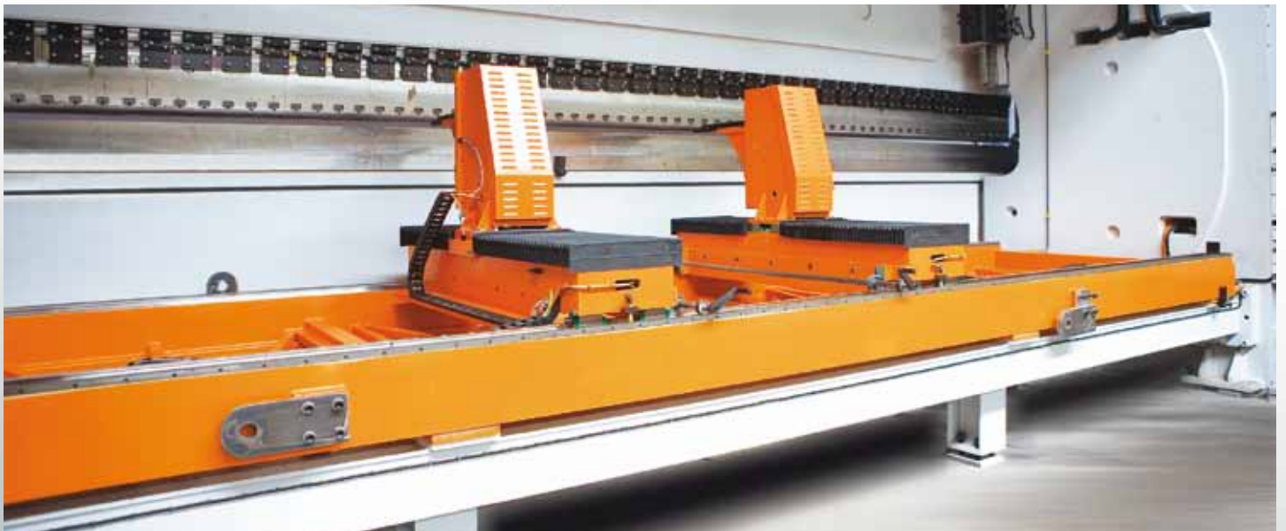
Heavy type 6 axes ( Y_1, Y_2, X_1, X_2, R_1, R_2 ) servo motorized back gauge.
