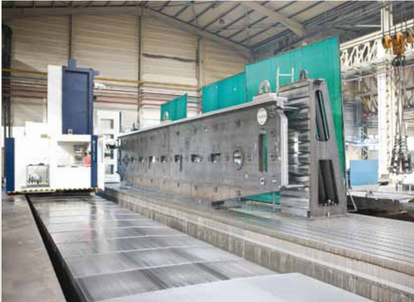
High precision CNC machining center 28 000 mm processing capacity in one piece.
