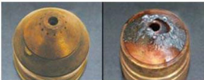
300 pierces at 50 mm (2") HPR400XD with PowerPierce technology
